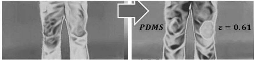
Figure R2. Infrared images on the clothes depending on the attachment of low emissivity material
